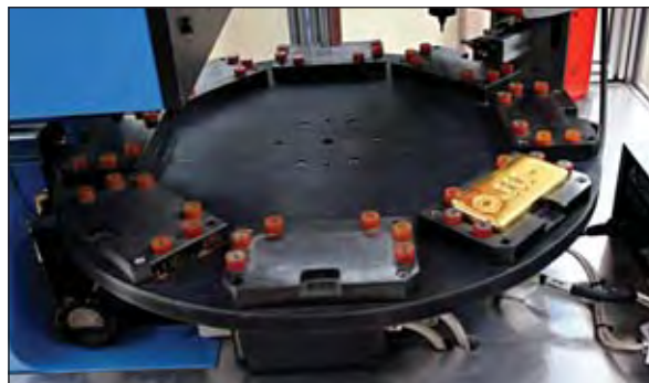
An automated unit stamps kilobars with the company's official stamp and other markings.
