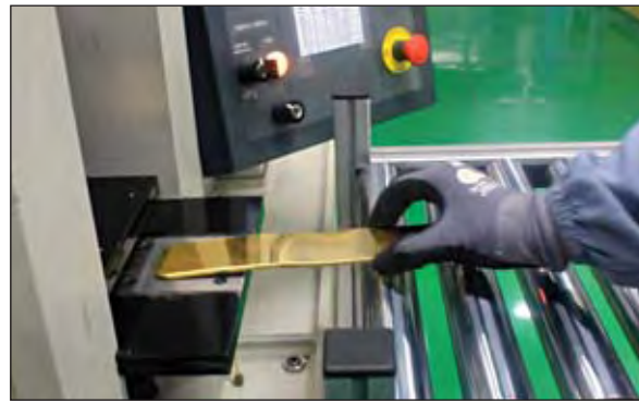
Producing flat gold strips for use in the manufacture of minted bars.
