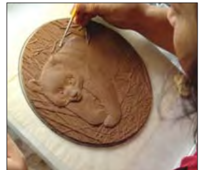
A plaster cast from which a Gold Panda design is transferred to minting dies.
