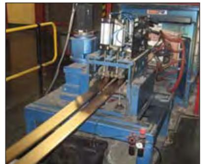
A continuous casting machine producing flat cast bars.
