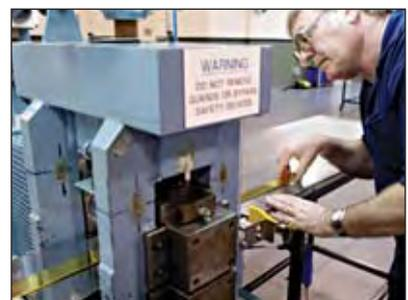
Rolling flat cast bars to the required thickness.
