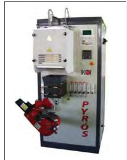
Continuous casting machines generate flat strips of gold for the manufacture of minted bars and coins.
