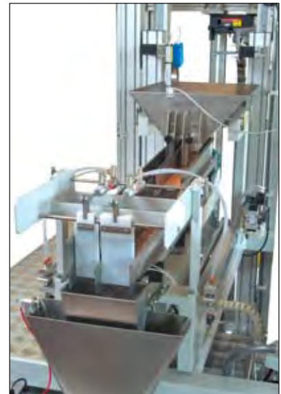
A "dosing" machine adds a small amount of wire clippings to each crucible or mould containing grains.
