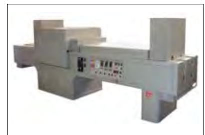
Annealing belt furnaces harden the blanks that are used to produce minted bars and coins.
