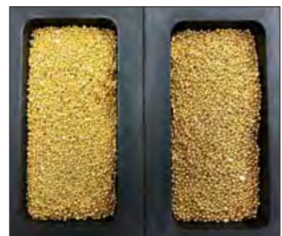
Graphite moulds containing an exact weight of gold grains and wire, prior to being melted in a Flameless Tunnel® Machine.
