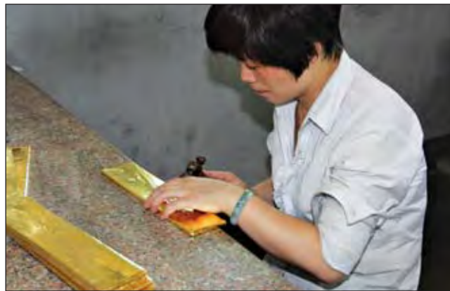
Manufacturing 3000 g bars at the refinery in Shanghai. The refinery in Luoyang also manufactures Shanghai Good Delivery bars as a separate company. The bars are marked with its own official stamp.
