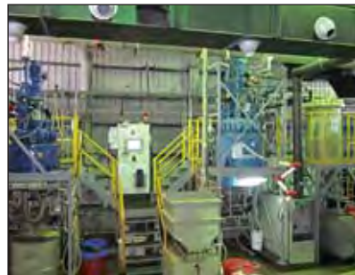
Gold refining relies mainly on the wet chemical chlorination process.
