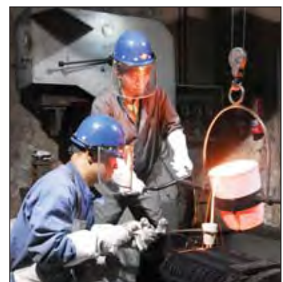
Pouring gold at the Zhongyuan Gold Smelter.
