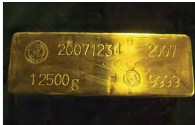
The year date has been applied to London Good Delivery 400 oz (12.5 kg) bars since 2007.
