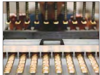
Manufacturing small cast bars at Metalor (Switzerland).
