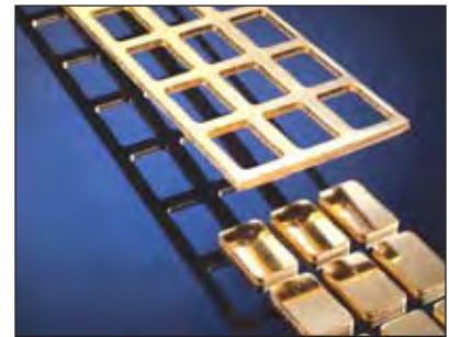
Minted bars are normally cut from a cast bar that has been rolled to a uniform thickness.
