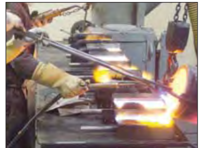
Most large cast bars are manufactured by pouring melted gold into an open mould.
