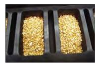
Kilobar moulds, containing exactly 1000 g of gold granules, prior to melting in an electric furnace.
